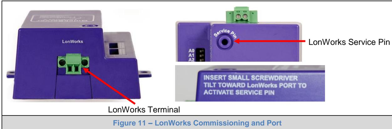
To commission the QuickServer LonWorks port, insert a small screwdriver in the commissioning hole on the face of the QuickServer's enclosure to access the Service Pin. See the instructions on the QuickServer as to which way to toggle the screwdriver during commissioning.
