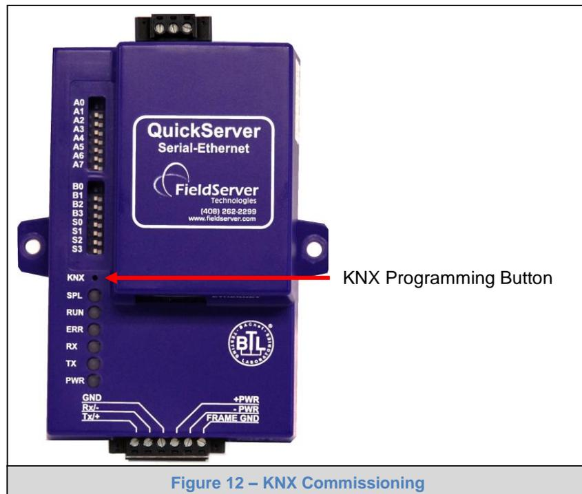
To commission the QuickServer as a KNX device in ETS Software, insert a small pin into the KNX commissioning hole on the face of the QuickServer to access the button.
