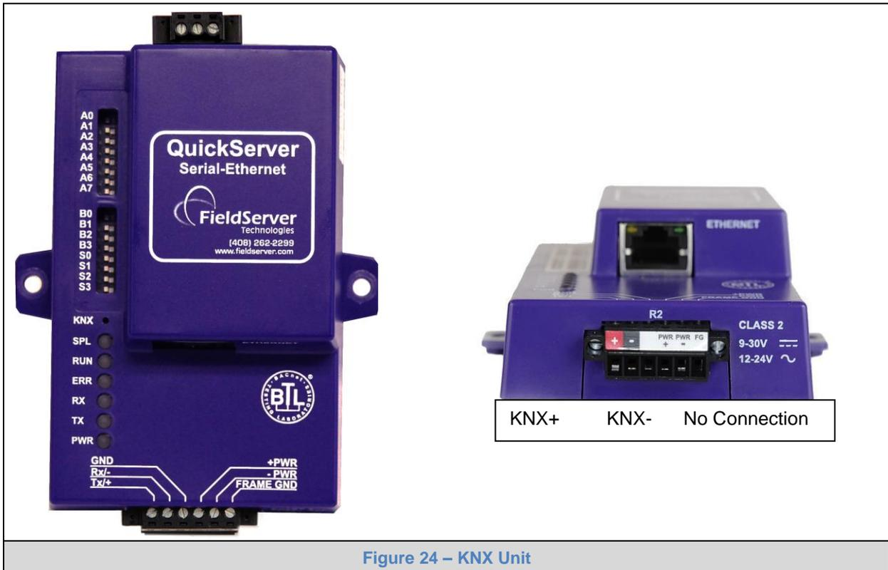
The KNX Connector consist of a KNX + and KNX- terminal. Each terminal corresponds to the red KNX+ and gray KNX- bus connections on a KNX bus.
